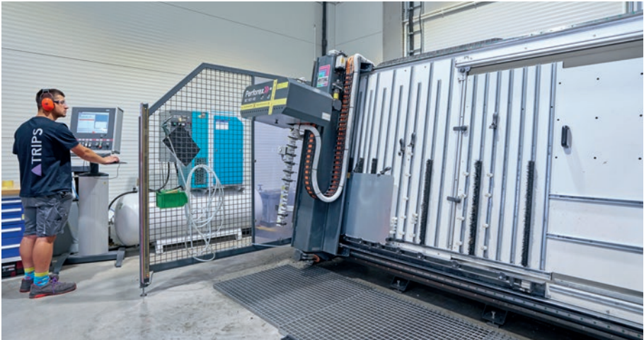
At the new plant of TRIPS Automatyka Polska, enclosures and panels can be machined automatically at the touch of a button using the Perforex machining centre from Rittal.
